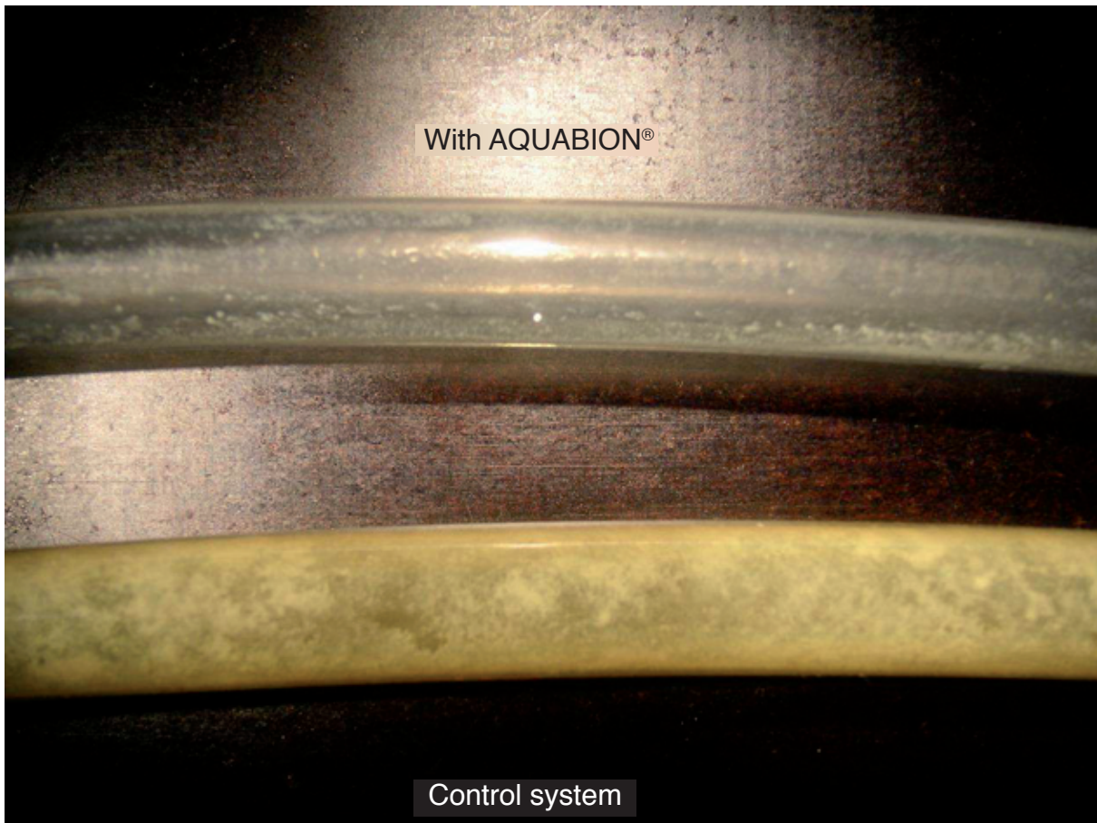
Figure 5: Macroscopic examination of the hoses from the system with AQUABION® (top) and the control system (below).
